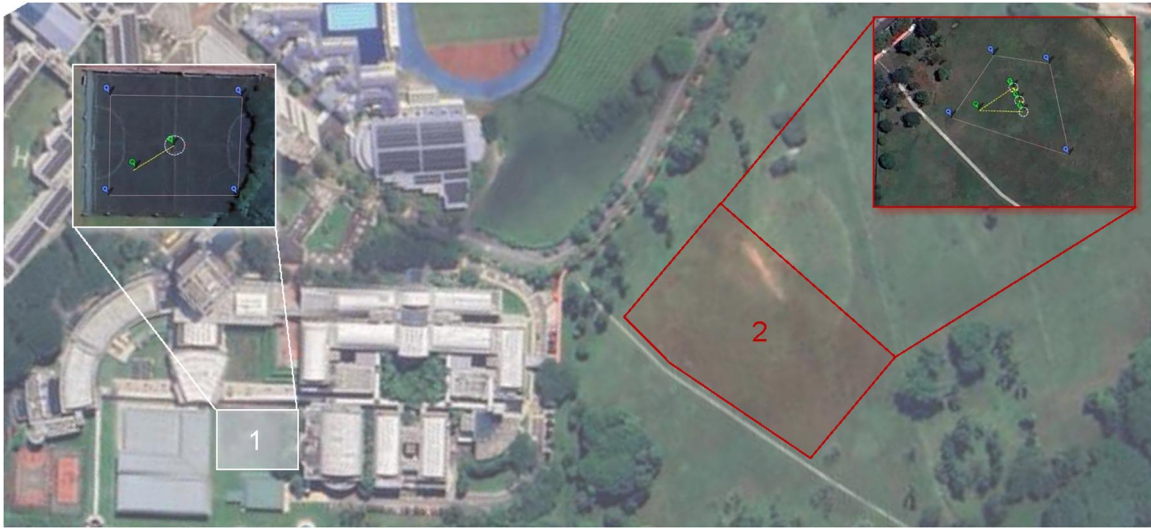
FIGURE 11 | Flight testing locations with planned autonomous mission waypoints (green) and geofences (blue): (1) netted futsal court; (2) outdoor field. [Color figure can be viewed at wileyonlinelibrary.com ]
