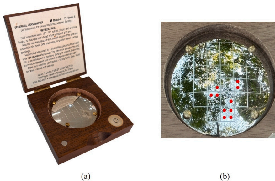
Fig. 7. (a) Forest densiometer model A, showing grid of 24 squares engraved upon the surface of a concave mirror; (b) example of forest densiometer quarter squares, reflecting mostly sky, counted—indicated by red dots: R12, 5th plot, taken on November 18, 2023.
